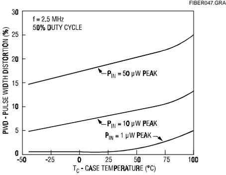
Fig. 3 Pulse Width Distortion vs Optical Input Power
