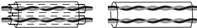
Figure 9 A double shielded twisted pair cable on the left and a single shielded twisted multipair cable on the right.
