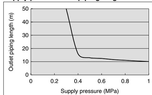
When the piping length is long and capacity is large due to a branch, install a speed controller (AS2051F-06, AS3001F-06, etc.) close to the A port of the VR51 in accordance with the below figure. Use the VR51 after adjusting properly to operate it.
