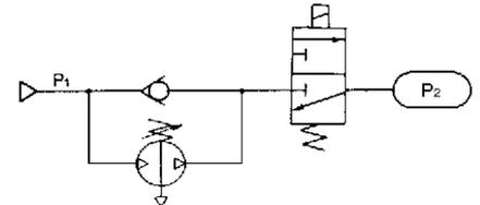
Initially, inlet pressure (P<sub>1</sub>) passes through the check valve, fills P<sub>2</sub>, and results in P<sub>1</sub> = P<sub>2</sub>.
