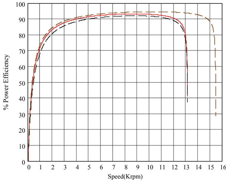
**Figure 15 – Improved Power Efficiency with Lower Winding Temperature**
