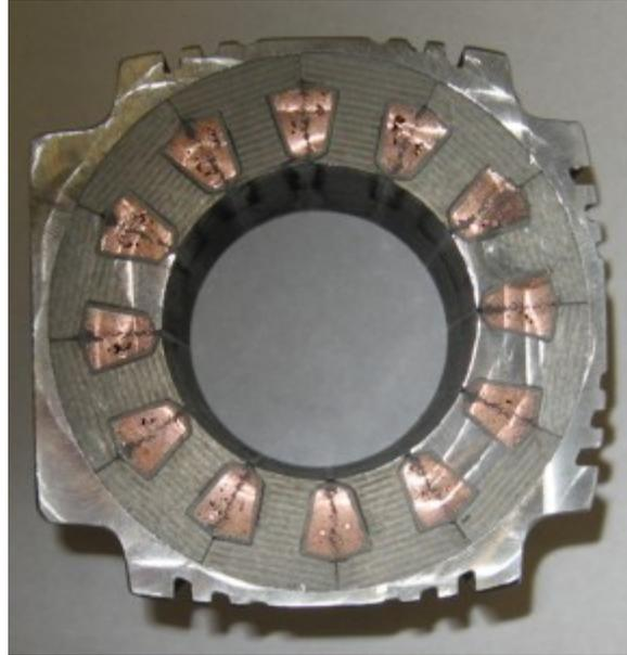
**Figure 11 – Cross-Section of Potted T-LAM Stator**
