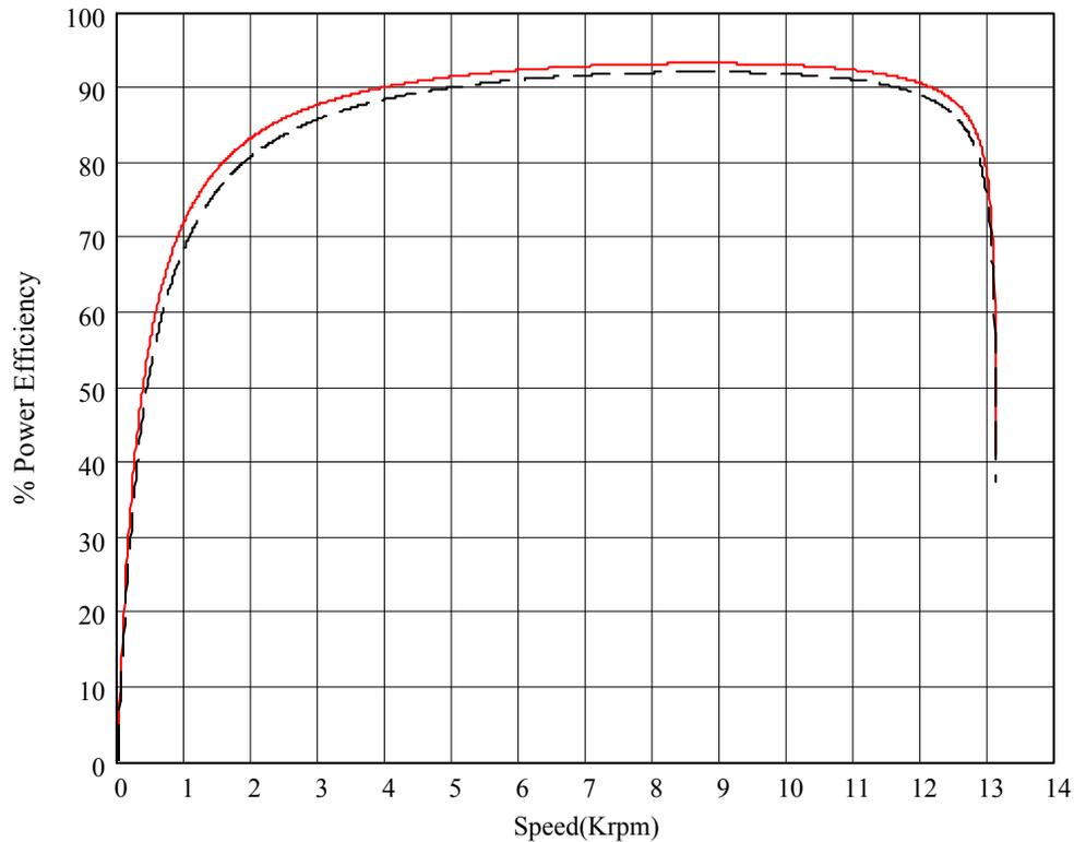
**Figure 9 – SLM90-238 Continuous Power Efficiency-Speed Curve**
