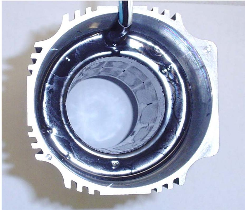
**Figure 10 – T-LAM Stator Potted with Thermally Conductive Epoxy**
