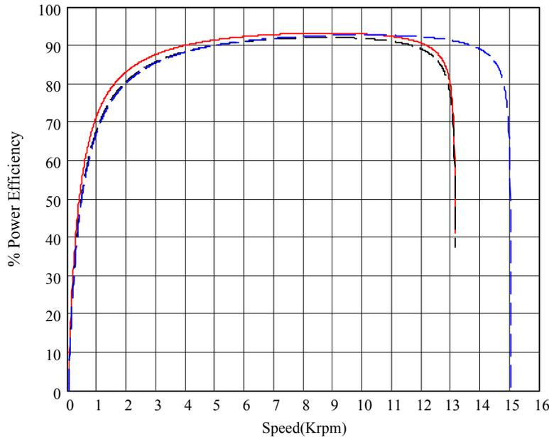
**Figure 14 – SLM90-238 Continuous Power Efficiency Curve**
