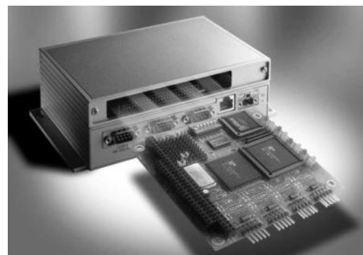
Extend I/O or Communication function by PC/104 extension
