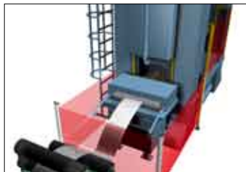
Perimeter guarding with reduced resolution combines light screens and mirrors to guard a machine, while allowing material to pass through.
