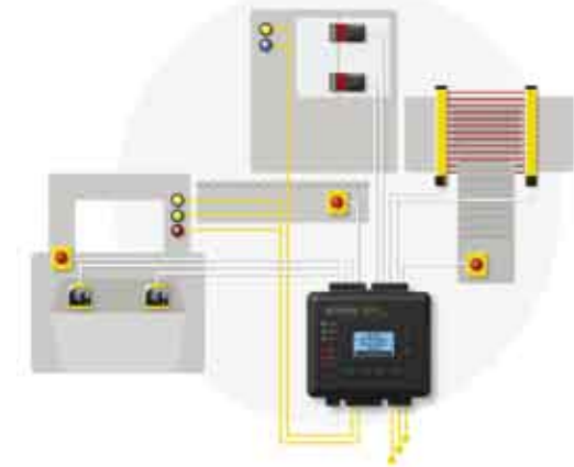
22 input terminals for monitoring safety and non-safety devices
