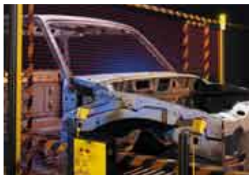
Controllers with muting suspend safeguarding during hazard-free times in the machine's cycle.
