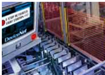
DeviceNet™ controllers can be integrated directly into a new or existing DeviceNet network, for non-safety monitoring of system.
