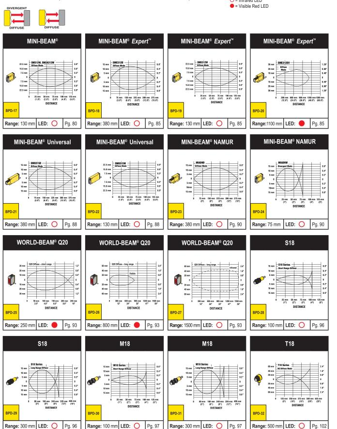
Diffuse Mode (Performance based on 90% reflectance white test card)
