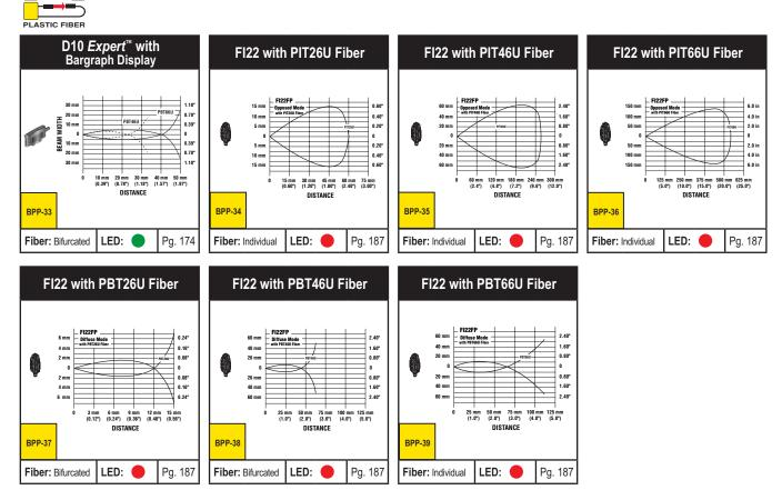
Plastic Fiber Optic Mode (Performance based on 90% reflectance white test card)
