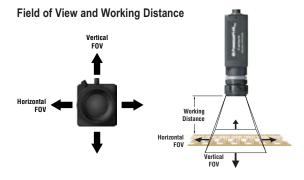
Sensor: The sensor contains the imager, microprocessors and I/O. The imager has an array of tiny light-sensitive cells that converts the target into an image.
