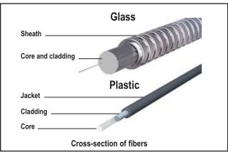
**Core** – Thin glass or plastic center of the fiber through which light travels.
