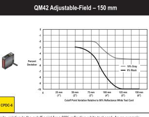
The percentage of deviation indicates a change in the cutoff point for either 18% gray or 6% black targets, relative to the cutoff point for a 90% reflective white test card. As an example, the cutoff point decreases 10% for a 6% reflectance black target when the cutoff point is 2000 mm using a 90% reflectance white test card. In other words, the cutoff point for the black target is 1800 mm.
