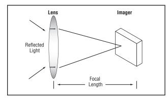
Angle of View: Angle of view indicates how much of the visual scene can be captured by the lens. It is determined by the focal length of the lens and how far away the camera is from the target.
