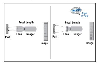
Working Distance: The distance from the camera to the target object under inspection.
