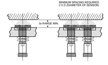
SENSORS MUST BE MOUNTED SUCH THAT SURROUNDING METAL IS NOT IN THE SENSING AREA.
