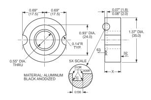
Kits include two mounting bolts and 0-Ring. Replacement 0-Ring is EE972-19306 (Equivalent to Parker # 2-116V709-90). Specify spacer height.
