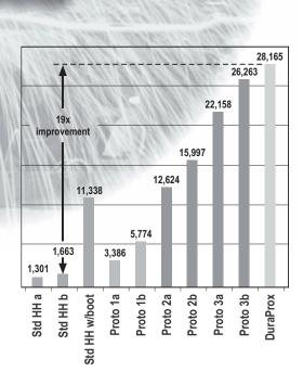
A wide range of materials were tested to determine optimal surface hardness and thermal characteristics necessary to survive the rigors of the automotive welding environment.
