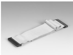
1701400972 HDD Cable, ATA 66/100, 82 cm + 15 cm
