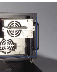
Hot-swap and redundant power supply
