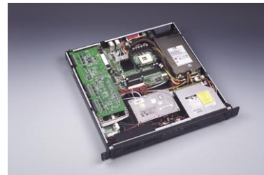
Supports one full-length 32-bit PCI expansion
