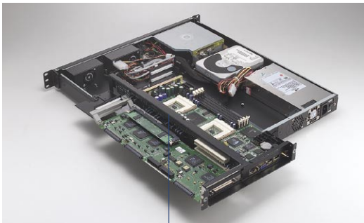
Butterfly backplane design supports two full-length 64-bit PCI expansions
