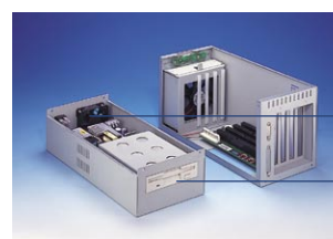
One 14-CFM cooling fan One 3.5" drive bay
