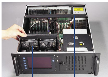
Two replaceable 84-CFM cooling fans Hold-down clamp
