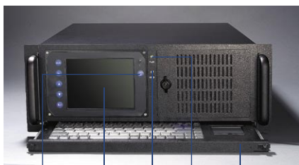
OSD power LCD Display LED HDD LED Power LED Slim type keyboard and touch pad
