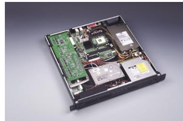
Supports one full-length 32-bit PCI expansion
