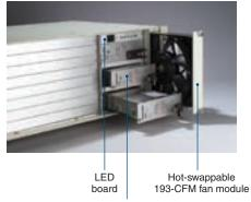
AC cPCI 500 W + 250 W redundant (2+1) power supplies
