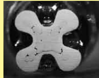
Crimp-cross section HARTING crimp profile
