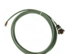
PLC Adapter Cable HMI-CAB-ST001 Connects to AGP3000/ST40x serial port with 9-conductor open-ended wires for connecting to third-party screw terminal devices.
