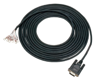
GP Multi-Link Cable (5m) CA3-CBLMLT-01 Connects a host controller to the AGP RS-422 port for multi-link (n:1) communication.
