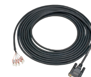
GP 2 Port Adapter Cable (5m) CA3-MDCB11 Connects Mitsubishi PLC to the AGP RS-422 port using 2-port adapter II (GP070-MD11).
