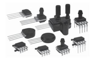
The pressure is on. The answer is here. No matter the need, Honeywell Sensing and Control (S&C) has the microstructure, pressure sensor solution. Our sensing element design consists of four piezoresistors galvanized with a thin, chemically etched silicon diaphragm. A pressure change will flex the mechanism, causing a strain in the diaphragm and the buried resistors. The resistor values will change in proportion to the stress
