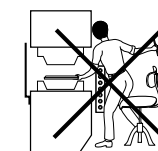
Penetration in danger zone over the barrier
