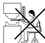
Penetration in danger zone under the barrier
