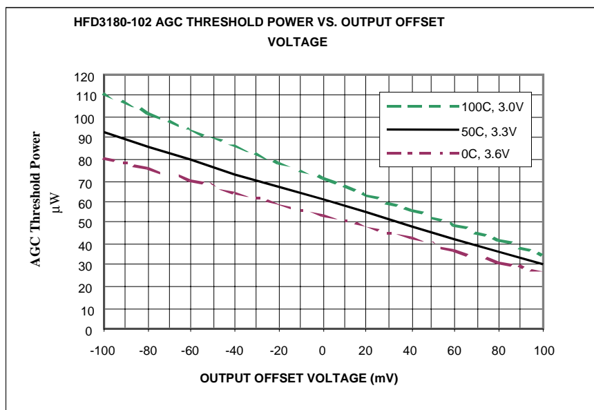
FIGURE 3: AGC THRESHOLD POWER VS. OUTPUT OFFSET VOLTAGE
