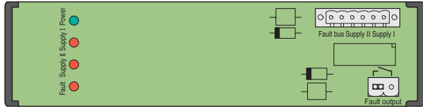
Figure 5 Fault Indication Board
