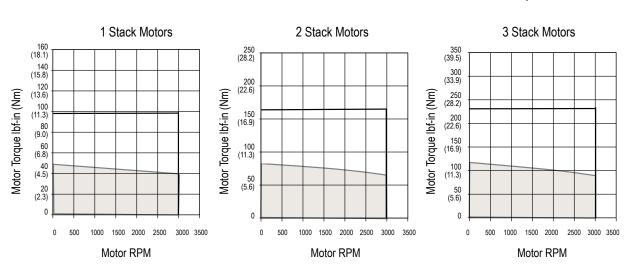
For gearmotors, divide speed by gear ratio; multiply torque by gear ratio and effciency. Efficencies: 1 Stage = 0.91, 2 Stage = 0.86 Test data derived using NEMA recommended aluminum heatsink 12" x 1/2" at 25°C ambient.
