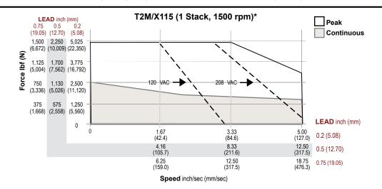
\*Test data derived using NEMA recommended aluminum heatsink 12" x 12" x 1/2" at 25°C ambient.
