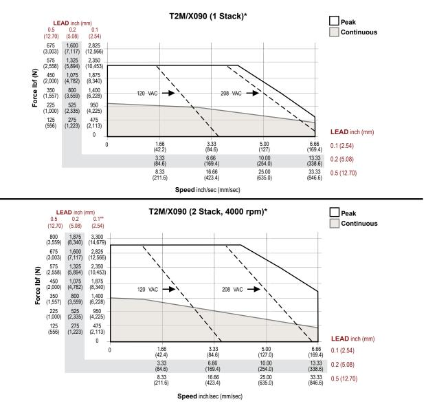
\*\*T2X peak force for 0.1 inch lead is 2700 lbf (12010 N). T2M peak force for 0.1 inch lead limited to 1620 lbf (7206 N).
