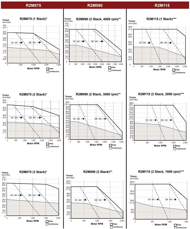
For R2G gearmotors, multiply torque by gear ratio and efficiency. Efficiencies: Divide speed by gear ratio; 1 Stage = 0.91, 2 Stage = 0.86 \*R2M075 test data derived using NEMA recommended aluminum heatsink 10" x 10" x 3/8" at 40°C ambient. \*\*R2M090 test data derived using NEMA recommended aluminum heatsink 10" x 10" x 3/8" at 25°C ambient. \*\*R2M115 test data derived using NEMA recommended aluminum heatsink 12" x 12" x 1/2" at 25°C ambient.
