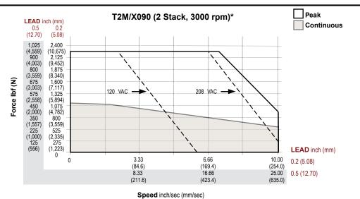
\*Test data derived using NEMA recommended aluminum heatsink 10" x 10" x 3/8" at 25°C ambient.
