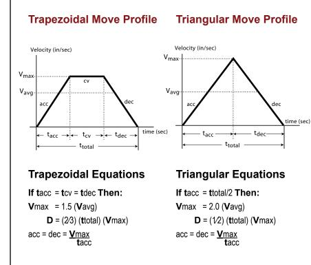
The second provides the necessary equations for determining the torque required from a linear or rotary application. For rotary applications this includes the use of reductions through belts or gears, and for linear applications, through screws.
