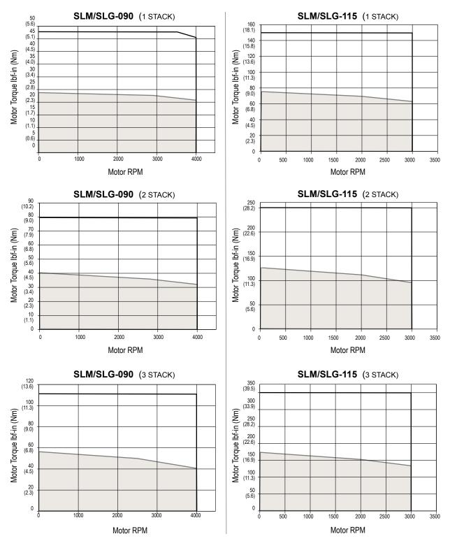
Test data derived using NEMA recommended aluminum heatsink 10" x 10" x 3/8" on SLM/SLG090 and 12" x 1/2" x 1/2" on SLM/SLG115 at 25°C ambient. For gearmotors, divide speed by gear ratio; multiply torque by gear ratio and effciency. Efficencies: 1 Stage = 0.91, 2 Stage = 0.86
