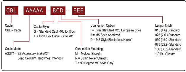
All Exlar cables rated IP65 when mated to actuator.
