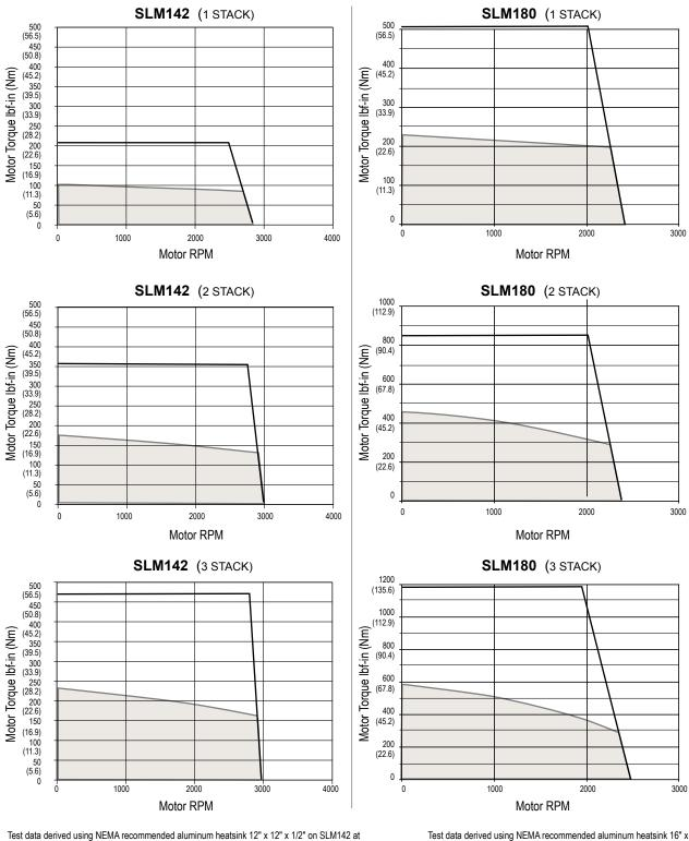
lest data derived using NEMA recommended aluminum heatsink 12" x 12" x 1/2" on 25°C ambient.
