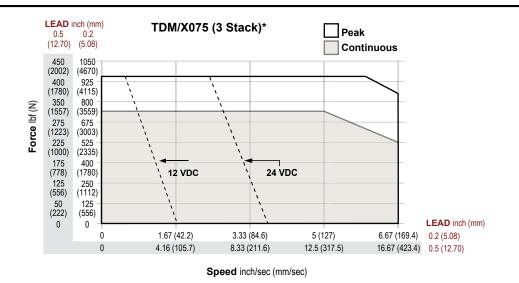
\*Test data derived using NEMA recommended aluminum heatsink 10" x 10" x 3/8" at 40°C ambient.
