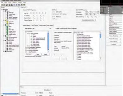
You can select up to four Tritex drive parameters to be monitored simultaneously.
