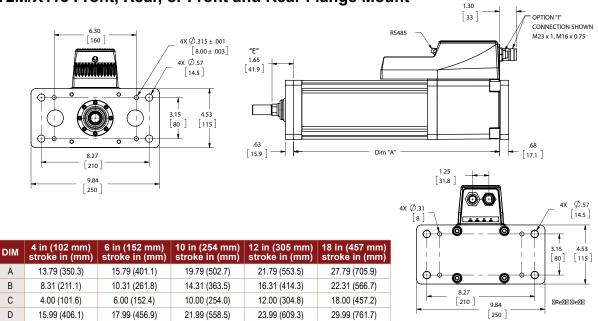
\* Add 2.33 inches to dimensions "A", "B" and "D" if ordering a brake. Add 1.77 inches to dimensions "A", "C" and "D" and dimension if ordering a splined  $\Delta$  main rod.
