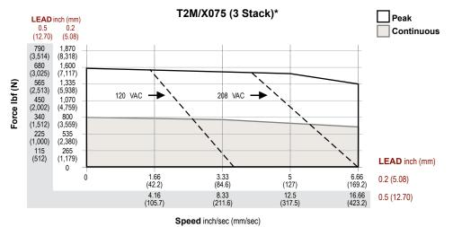
\*Test data derived using NEMA recommended aluminum heatsink 10" x 10" x 3/8" at 40°C ambient.
