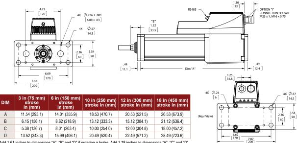
Add 1.61 inches to dimensions "A", "B" and "D" if ordering a brake. Add 1.78 inches to dimensions "A", "C" and "D"
