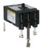
Rear connecting studs are designed to allow rear termination in applications, such as control panels where wire gutter space may be limited. The studs can be bolted directly to the bus bars or lugs can be attached to the studs. Long and short studs should be alternated on adjacent poles to assure proper electrical clearance. These studs are not UL Listed.
