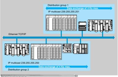
The Global Data service ensures data exchanges in real time between stations belonging to the same distribution group. It is used to synchronize remote applications, or share a common database among several distributed applications.
