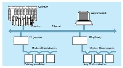
Modbus serial line (Modbus SL) protocol is a world-wide de facto standard. Is simplicity, reliability and low cost enabled it to have today, probably the most impotant installed base of communicating industrial products.
