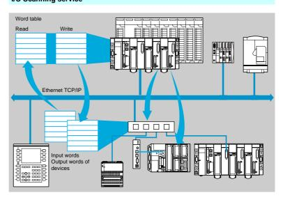
The I/O Scanning service can be used to manage the exchange of distributed I/Os on the Ethernet network after a simple configuration operation, with no need for special programming
