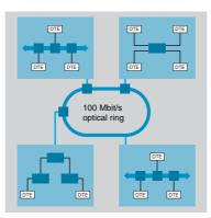
Switches (see "Cabling system" page 2/32) are used to increase the limits of architectures based on hubs or transceivers, by separating collision domains. Higher layer communication is provided between the ports, and collisions at link layer are not propagated (filtering). They therefore improve performance by better allocation of the pass band due to the reduction of collisions and the network load.
