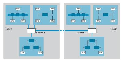
Switch used to isolate several collision domains (reduction of the network load in order to improve performance).
