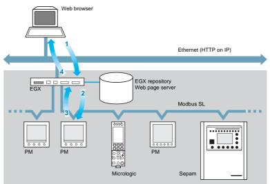
The EGX gateway uses HTML language for serving the Web pages containing dynamic values associated with the products on the Modbus SL link, and is thus compatible with all Web browsers. This mechanism is totally transparent for the user.
