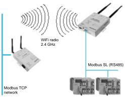
Serial Modbus to Modbus TCP connection
