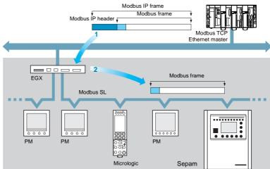
When accessing product data on the Modbus SL link, via Modbus messaging, the gateway has no added value other than translating addresses, encapsulating and unencapsulating Modbus frames, whatever function code is used. The gateway thus provides products on the Modbus SL serial link with the Ethernet pass band and a multi-master operating capability. The latter function is also effective when the Modbus master is connected directly to one of the two Modbus SL
