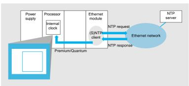
The time synchronization service is based on the NTP (Network Time Protocol) which is used to synchronize the time of a client or a server on Ethernet TCP/IP from a server or another reference time source (radio, satellite, etc).
