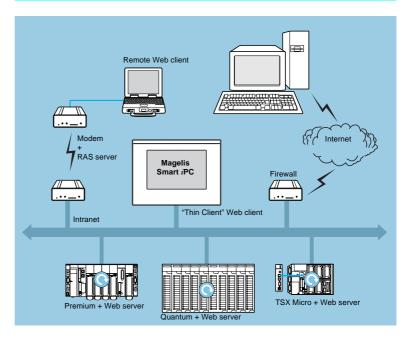
In addition to standard Web services, FactoryCast modules (see selection table on page 2/3) support the following functions:
