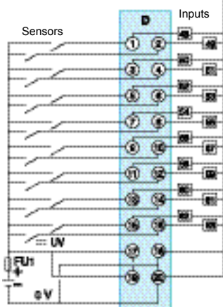
FU1: 0.5 A fast-blow fuse
