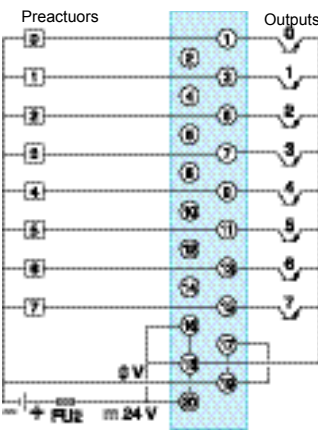
FU2: 16 A fast-blow fuse
