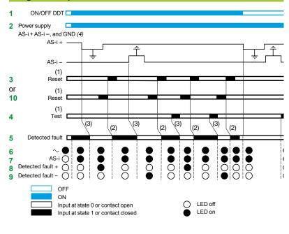
(1) 30 ms min. (2) 15 ms (3) 20 ms (4) Warning: the ground fault detector will work only if the ground (GND) terminal is connected.
