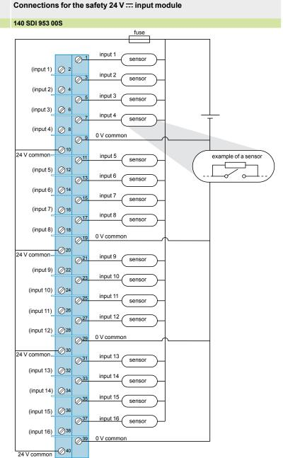
**Power supply:** 24 V ..... **Fuse:** 1 A fast-blow fuse. **Internal input impedance:**  $3675 \text{ k}\Omega$ . **Pull-up resistor at the sensor power supply** (in the example of a sensor with volt-free contact):  $15 \text{ k}\Omega$ .
