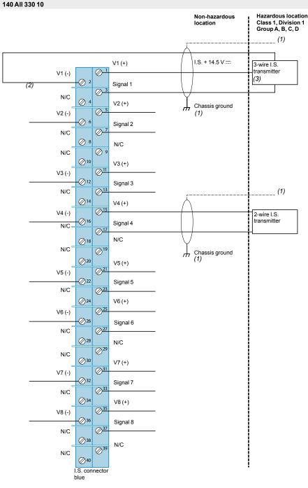
Only shielded twisted pair cables should be used for connection to ground at the module end (on specially-designed screws on the rack).
