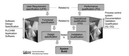
UAG uses ISA 88 standard terminology for batch control and supports the GAMP methodology for creating an automation system. The use of these two standards is a key element to achieve process validation.
