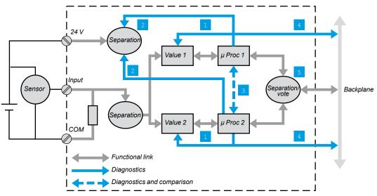
Each input channel uses a unique interface circuit and 2 independent inputs.
