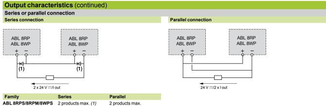
Note: Series or parallel connection is only recommended for products with identical references.
