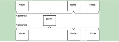
When a Modbus device, such as a programming terminal, operator interface or third-party computer, requires access to data from a Modbus Plus network, a BM85 Modbus Plus bridge must be used. The BM85 has four Modbus-compatible RS 232 serial ports, enabling a Modbus master or Modbus slave to connect to a Modbus Plus network. The bridge connections allow data exchanges between Modbus devices and with the entire Modbus Plus network.
