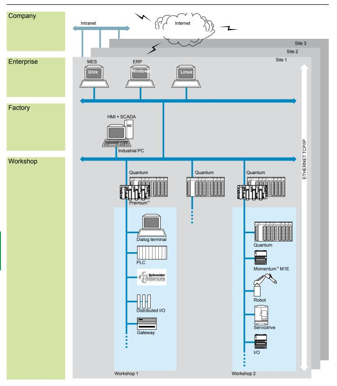
MES: Manufacturing Execution System (production management system) ERP: Enterprise Resource Planning (integrated management software packages) HMI/SCADA: Human/Machine Interface/Supervision Control And Data Acquisition Gateway: Bridge to sensor/actuator bus, to installed base network, field bus, etc.
