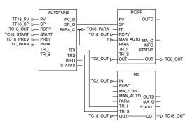
Example: PID controller with MS manual control
