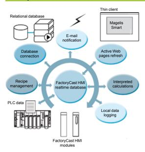
FactoryCast HMI Web services are integrated in the Web server modules embedded in the Modicon Premium<sup>™</sup> and Quantum automation platforms.
