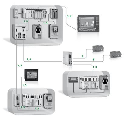
Key: 1, 3: Straight copper cables 2, 4: Crossed copper cables 8: Cables with IP 67 connector See pages 6/48 and 6/49.
