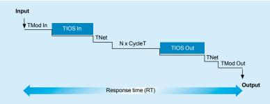
□ TMod In and TMod Out: Response time of the read/written device, excluding the electrical transit time at the input/output (TMod depends on the device, usually between 1 and 8 ms).
