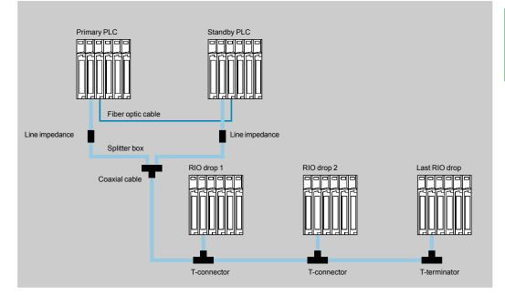
The Hot Standby system also accepts a redundant RIO cable topology. The two coaxial cables, from the two **140 CRP 932 00** head-end adaptors, on each of the two PLCs, are connected to the redundant RIO cable by two separate **MA 0186 100** splitter boxes.
