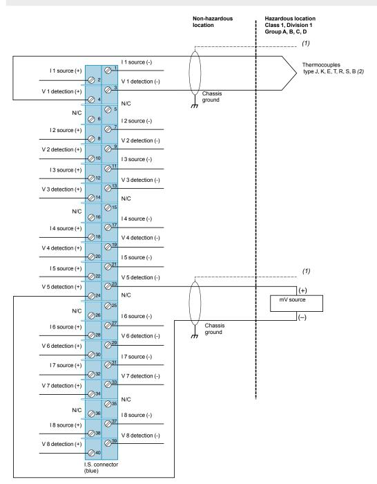
(1) Only shielded twisted pair cables should be used for connection to ground at the module end (on specially-designed screws on the rack).
