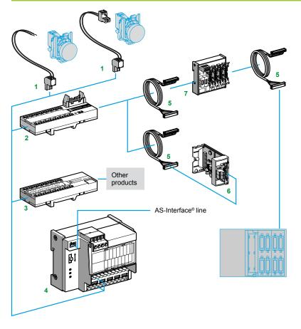
Tego Dial offers a range of interface components and cabling accessories that simplify connection of control and signalling units to PLCs, buses and other products. This range includes in particular:
