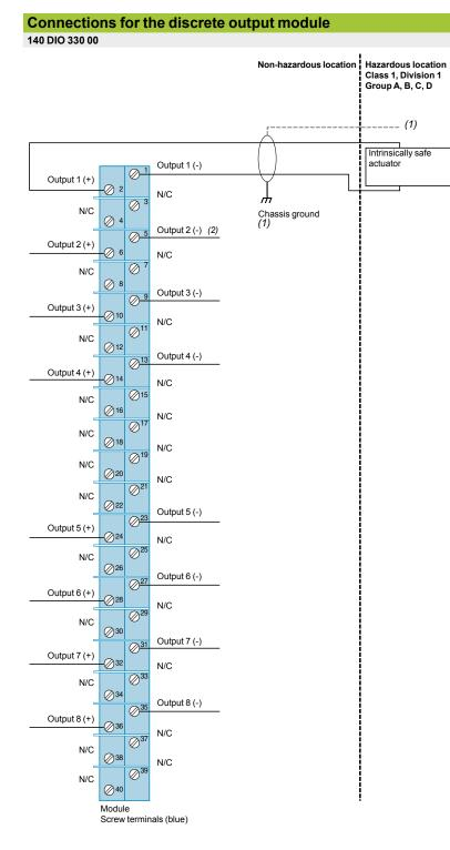
(1) Only shielded twisted pair cables should be used for connection to ground at the module end (on specially-designed screws on the rack). (2) The (-) outputs are connected together internally.
