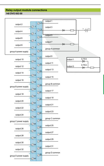
**Note:** When connecting 2 outputs in parallel, a diode is required for each point. See detailed diagram above.
