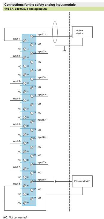
Internal input impedance:  $287 \Omega$ .
