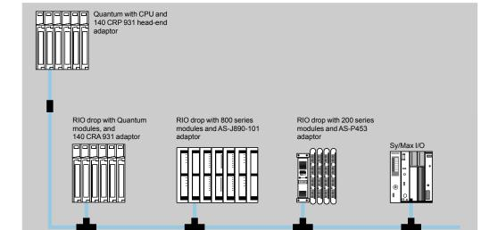
The RIO architecture uses coaxial cabling, and provides long distance capability up to 4572 km with a CATV cable, or longer with an optional fiber optic cable. It is a high-performance network, operating at 1.544 Mbps, providing a high I/O data throughput.
