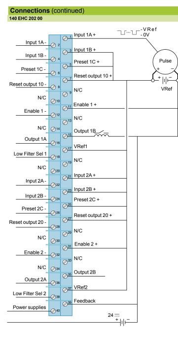
Basic wiring diagram showing non-differential connections for:
