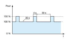
The ABL 8RPS/RPM/WPS Universal range of Phaseo power supplies has a power reserve, allowing them to supply the application with energy up to 1.5 times the nominal current at the intervals illustrated by the graph opposite.
