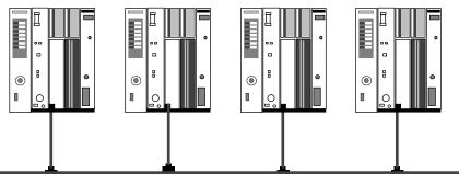
The original Sy/Max I/O wiring remains intact. Because the I/O is now on a Quantum RIO network, they can take advantage of its 1.544 Mbps data transfer rate with 16-bit CRC.
