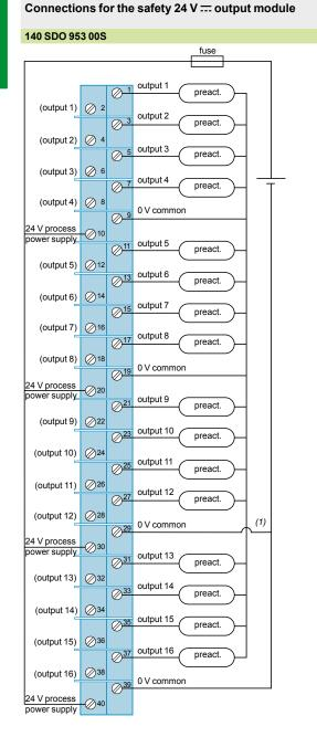
Power supply: 24 V ..... Fuse: max 10 A fast-blow. Preact: preactuator.
