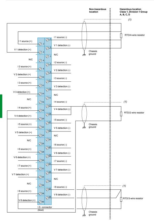
(1) Only shielded twisted pair cables should be used for connection to ground at the module end (on specially-designed screws on the rack).
