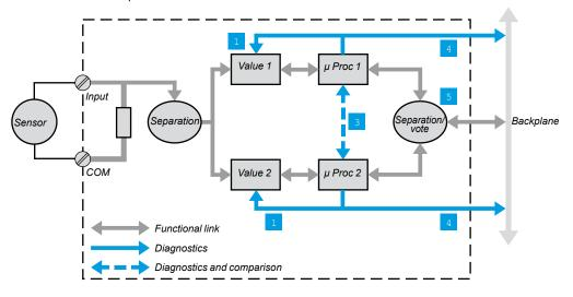
The interface on the process side consists of 8 independent isolated input channels. Each input is acquired by 2 identical circuits.
