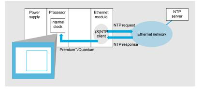
The time synchronization service is based on the NTP (Network Time Protocol) that is used to synchronize the time of a client or a server on Ethernet TCP/IP from a server or another reference time source (radio, satellite, etc.).
