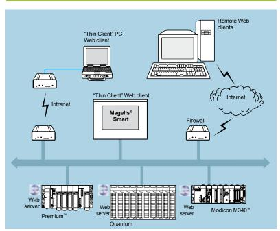
The predefined "Rack Viewer" PLC diagnostic function and the "Data editor" read/ write functions are supported by Ethernet TCP/IP modules (1) in the following Modicon automation platforms:
