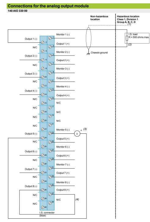
(1) Only shielded twisted pair cables should be used for connection to ground at the module end (on specially-designed screws on the rack).
