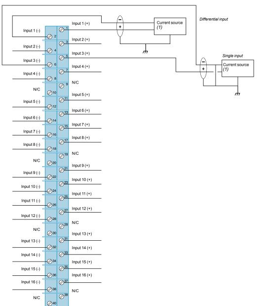
Use shielded or unshielded connection cables. In noisy environments, the use of twisted shielded cable and STB XSP 3000 grounding kits with STB XSP 3010/3020 terminal blocks is recommended, see page 4/55. The shielded cable must be connected to the machine ground at the signal source end.
