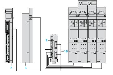
The motor starter is connected to an APP 1Ce 7 module using an APP 2CX 8 adaptor plate and an APP 2AH40H060 10 cable.
