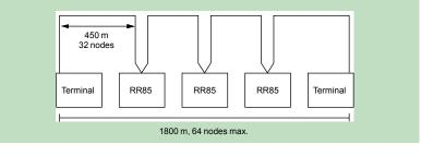
If an application requires more than 64 nodes, a BP85 Modbus Plus bridge can be used to connect two Modbus Plus networks. Bridge devices can be used to interconnect network segments to achieve maximum performance.
