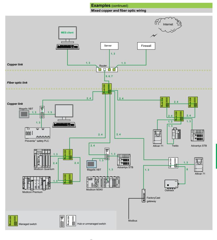
Key: 1, 3: Straight copper cables 2, 4: Crossed copper cables 5, 6, 7: Fiber optic cables 8: Cables with IP 67 connector
