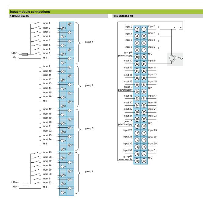
Discrete I/O modules Input module connections
