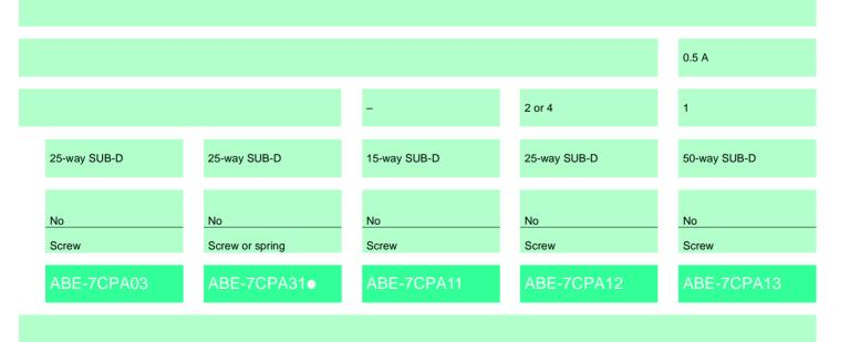
Telefast<sup>®</sup> 2 pre-wired system Passive connection sub-bases
