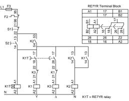
A No galvanic insulation between supply terminals A1, A2, B1, B2 and control input Z2. This terminal must therefore never be used (factory setting).
