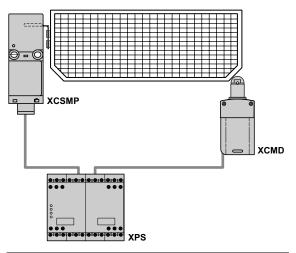
Locking by operating key and actuation in positive mode with a safety relay
