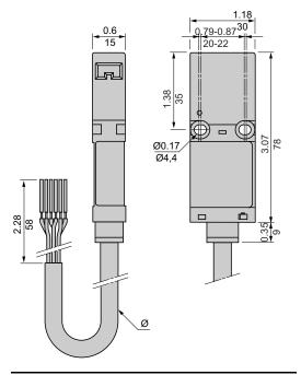
$\varnothing$ : 0.29 in (7.6 mm); Length 6.6 ft (2 m) , 16.4 ft (5 m), or 32.8 ft (10 m)
