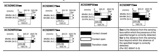
The contact status and magnet positions above are for when non-ferrous and non-ferromagnetic materials are used for the mounting surface and mounting hardware. Using ferrous and ferromagnetic materials may reduce the published sensing distances.
