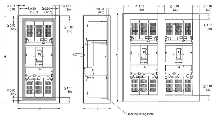
Minimum Enclosure Dimensions for Thermal Requirements
