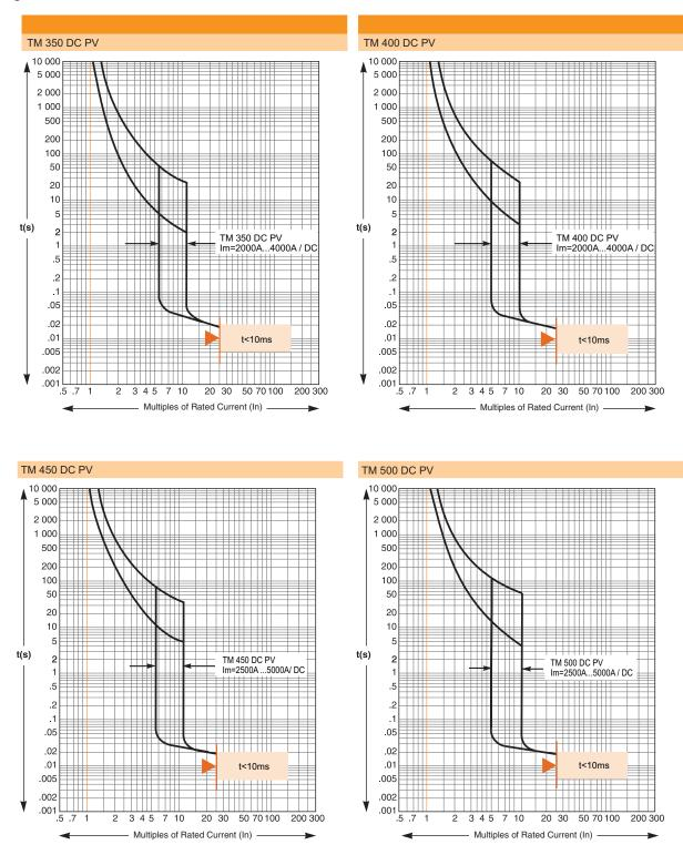
Figure 18: U-Frame 350–500 A DC Photovoltaic Circuit Breakers
