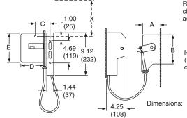
Refer to NEC Article 430-10 for minimum dimension X from circuit breaker top mounting hole to wall or barrier to ensure adequate wire bending space.
