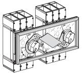
Interlocking with Rotary Handles (S32621)
