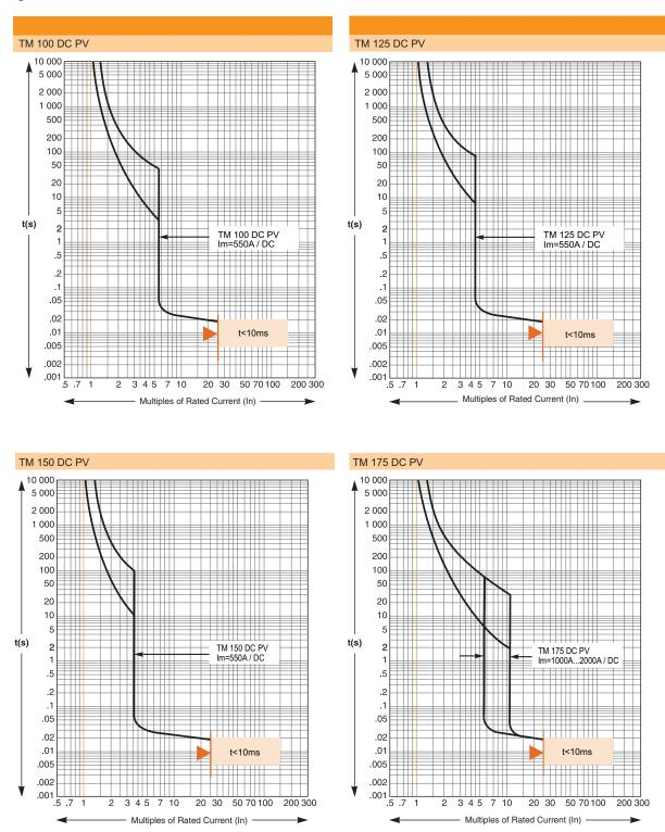
Figure 16: T-Frame 100–175 A DC Photovoltaic Circuit Breakers
