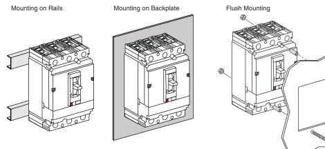
U-Frame Circuit Breakers (4 Mounting Screws)
