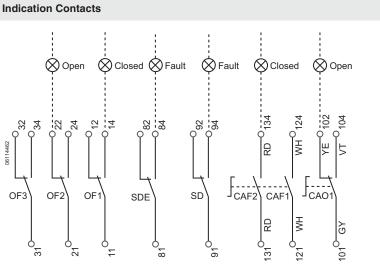
The diagram is shown with circuits de-energized, relays in normal position, and all devices open, connected, and charged.
