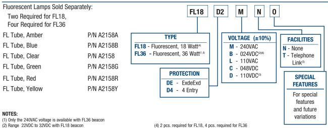
(3) Range 100VDC to 135VDC with xenon beacons (inclusive of  $\pm$ 10%). FL18 is 100VDC to 150VDC inclusive of  $\pm$ 10%.
