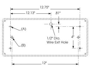
(A) Drill 0.20" Dia. holes (4) for top mounting or Drill 0.28" Dia. holes (4) for bottom mounting
