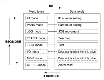
As shown above, 6 modes are available. (I/O mode and MON mode do not function with this driver.) When the communication mode is started by the teaching box, a menu can be selected with [ESC/MODE]. Select the mode indication LED for the mode to be implemented (all mode indication LEDs turn Off in the ID mode) and press [RET] to start each mode.
