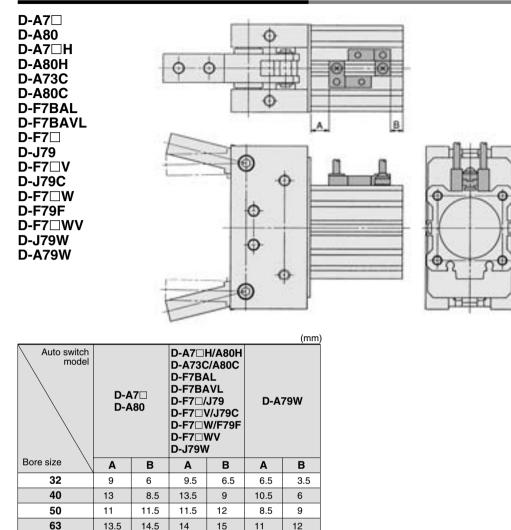
Note) The actual mounting position should be adjusted after confirming the auto switch performance.
