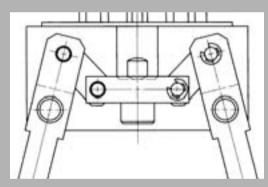
The toggle mechanism that activates when the finger closes realizes strong and stable gripping force. The mechanism also holds workpiece even when pressure drops.
