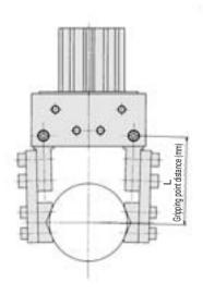
· Indication of effective gripping force The effective gripping force shown in the graphs to the right is expressed as  ${\bf F},$  which is the thrust of one finger, when both fingers and attachments are in full contact with the workpiece as shown in the figure below.
