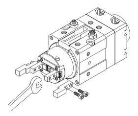
When mounting attachments on fingers, support the fingers with a tool such as a spanner to prevent them from twisting. Refer to the table on the right for the tightening torques of finger mounting
