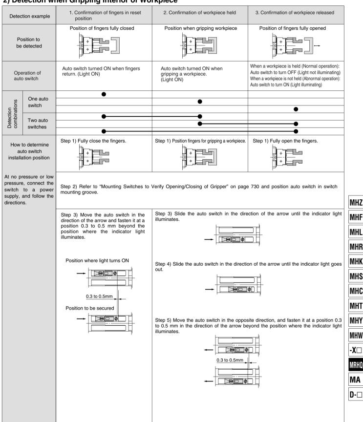
Note) • It is recommended that gripping of a workpiece be performed close to the center of the finger stroke.
