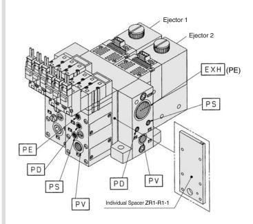
PV: Air pressure supply port PS: Pilot pressure supply port PD: Release pressure supply port PE: Pilot pressure exhaust port **EXH:** Common exhaust port V: Vacuum Port
