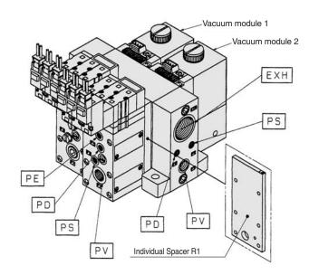
PV: Vacuum pressure supply port PS: Pilot pressure supply port PD: Release pressure supply port PE: Pilot pressure exhaust port **EXH:** Common exhaust port V: Vacuum Port
