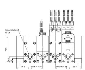
PV: Air pressure supply port PS: Pilot pressure supply port PD: Release pressure supply port PE: Pilot pressure exhaust port
