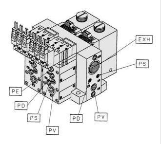
PV: Vacuum pressure supply port PS: Pilot pressure supply port PD: Release pressure supply port PE: Pilot pressure exhaust port **EXH:** Common exhaust port
