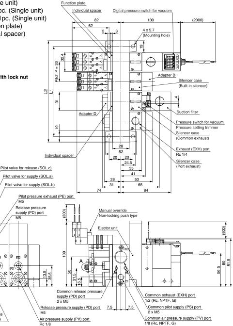
1 The common exhaust port (EXH.) is also used as the pilot pressure exhaust (PE) port of the pilot valve. Use while the port is open to the atmosphere.
