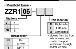
Note) The thread ridge shape is compatible with the G thread standard (JIS B 0203), but other shapes are not conforming to ISO16030 and ISO1179.
