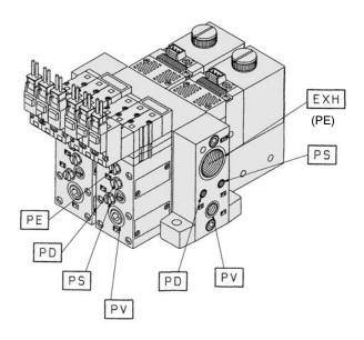
PV: Air pressure supply port **PS:** Pilot pressure supply port PD: Release pressure supply port **PE:** Pilot pressure exhaust port **EXH:** Common exhaust port V: Vacuum Port
