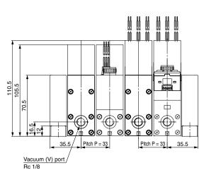
PV: Air pressure supply port **PS:** Pilot pressure supply port PD: Release pressure supply port
