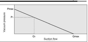
Flow characteristics are expressed in ejector vacuum pressure and suction flow. If suction flow rate changes, the vacuum pressure will also be changed. Normally this relationship is expressed in ejector standard use. In graph, Pmax is max. vacuum pressure and Qmax is maximum suction flow. The values are specified according to catalog use. Changes in vacuum pressure are expressed in the below order.
