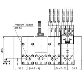
PV: Vacuum pressure supply port **PS**: Common pilot pressure supply port PD: Common release pressure supply port
