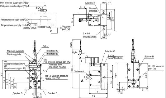
A: Release flow rate adjusting needle with lock nut
