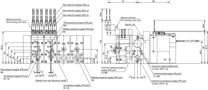
\* 1 The common exhaust port (EXH.) is also used as the pilot pressure exhaust (PE) port of the pilot valve. Use while the port is open to the atmosphere.
