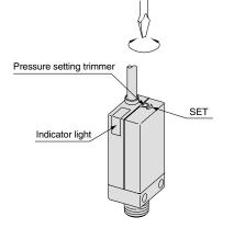
•When using the switch to confirm correct absorption, the vacuum pressure is set to the minimum value to reliably absorb. If the value is set below the minimum, the switch will be turned ON even when adsorption has failed or is insufficient. If the pressure is set too high, the switch may not operate stably even though it may absorb correctly.
