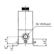
Note) \*1 Dimensions for mounting bracket C Bracket C part no. : P3270155#1 (Standard accessory)
