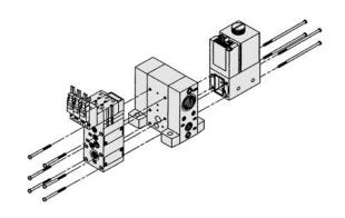
**Mounting Thread Parts List for Unit Combination**
