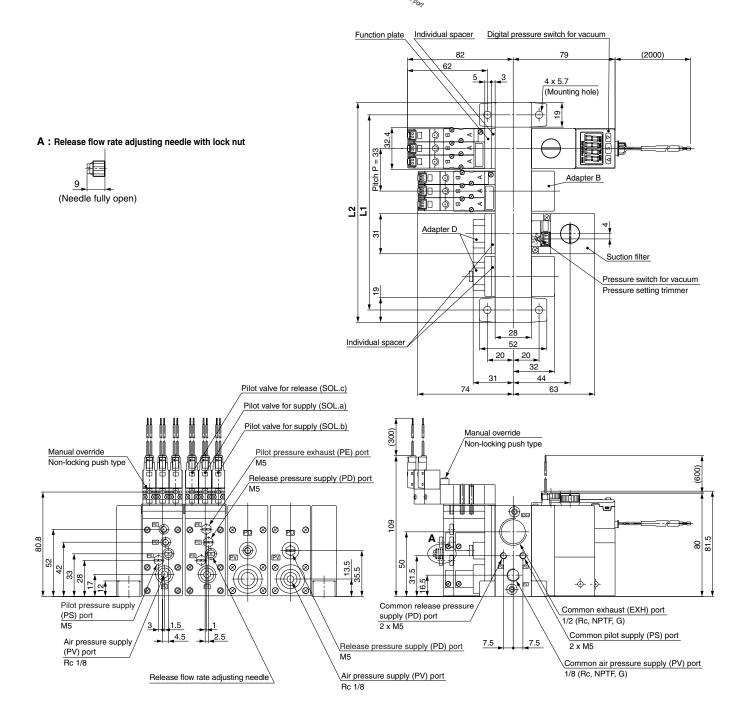
1 The common exhaust port (EXH.) is also used as the pilot pressure exhaust (PE) port of the pilot valve. Use while the port is open to the atmosphere.
