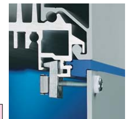
3 Spacer trim For installed equipment flush with the frame section. For front panel thickness up to approx. 3.5 mm (0.14").
