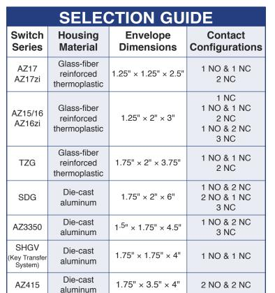
2 KEYED INTERLOCK SWITCHES WITH SOLENOID LATCHING
