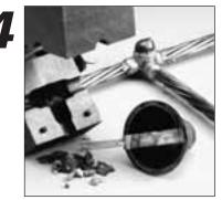
Open the mold and remove the expended steel cup – no special disposal required
