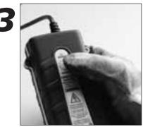
Press and hold control unit switch and wait for the ignition
