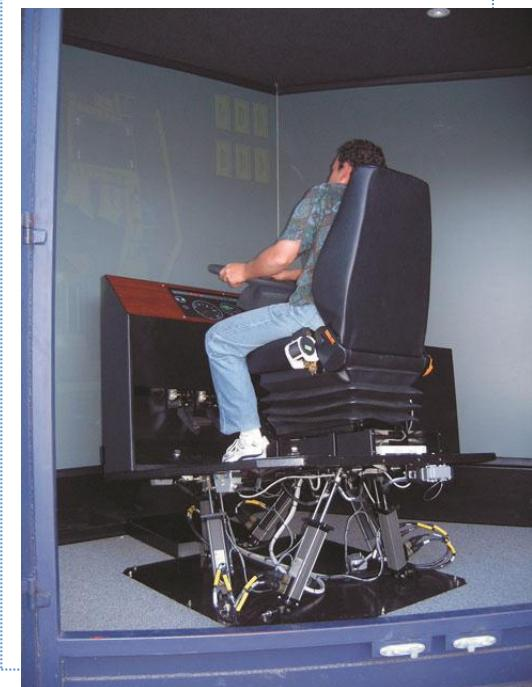
**Exlar Solution:** Six Exlar GSM20 actuators are used in the ThoroughTec mining equipment simulators. Two other families of linear actuators, the GSX Series and FT Series actuators are also available and offer varying stroke lengths, speeds, forces, and other mechanical
