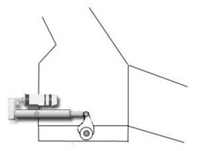
Drawing of Exlar's FT60 actuator installed on the coal diverter gate.
