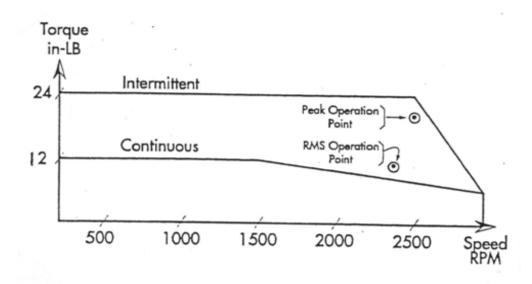
Figure 2, Motor's Intermittent and Continuous Torque-Speed Curves
