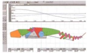
The program Working Model from MSC Software, Santa Ana, Calif., simulates the animatronic whale's motion and joint forces.
