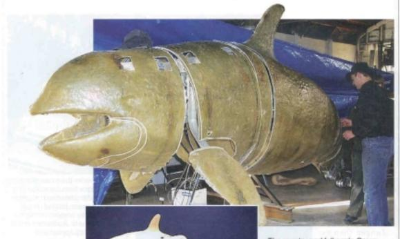
helped integrate the actuators and refine the 3D CAD model. The CAD model produced both engineering drawings and DXF files for NC machining of the various parts.
