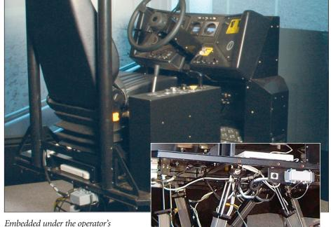
Embedded under the operator's station, Exlar SR21 linear actuators create 6-axis motion that mimics what would be the real-life reaction to a trainee's actions. Note that with no external motors, the entire assembly is clean and simple.
