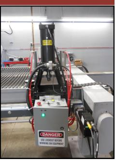
Exlar's Tritex II rotary actuator installed on automated riveting machine.
