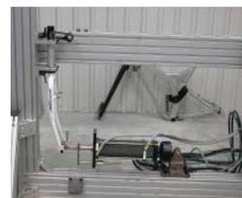
Exlar Actuators ideal for incorporation into strength testing
