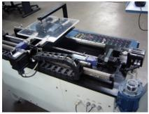
of what responses should be generated from the machine under ideal settings. Students learn how to adjust the CNC parameters as well as the velocity, torque and acceleration settings of the SmartMotor and PID parameters of the controller. The resulting adjustments can then instantly be compared to the input, allowing as little difference between the output and input as possible the minimize overshoots.
