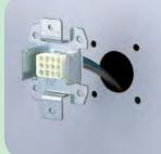
Drill the holes on the machine to attach the mounting connector and bracket.
