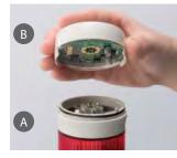
Affix the transmitter adaptor (A) on the Signal Tower and fasten it with the center screw. Then simply attach the transmitter to the bracket. (Some applications don't require additional wiring.)
