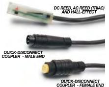
There are 10 sensing choices: DC reed, form A (open) or form C (open or closed); AC reed (Triac, open); Hall-effect, sourcing, PNP (open); Hall-effect, sinking, NPN (open); each with either flying leads or QD (quick disconnect). Commonly used to send analog signals to PLC (programmable logic controllers), TLL, CMOS circuit or other controller device. These switches are activated by the actuator's magnet.
