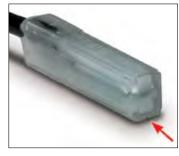
A THE NOTCHED FACE OF THE SWITCH INDICATES THE SENSING SURFACE AND MUST FACE TOWARD THE MAGNET.
