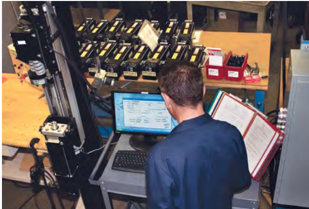
Functional unit testing for hundreds of cycles quantifies stroke, length, torque under no load, input current vs force standard deviation.
