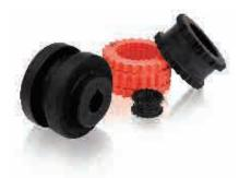
Three-way flexing action handles shock, vibration and misalignment. The ABB Dodge D-Flex<sup>™</sup> coupling features moulded, non-lubricated, interchangeable elastomeric sleeves of EPDM, neoprene Hytrel. Its three-way flexing action accommodates torsional, angular and parallel misalignment, as well as axial end float.
