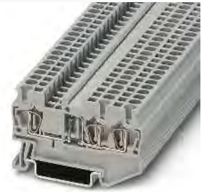
0.5 A, diode terminal block, 1N 4007 (1300 V/0.5 A), 3 connections
