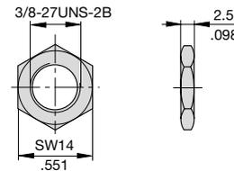
This is a metric design and millimeter dimensions take precedence ( $\frac{mm}{inch}$ )
